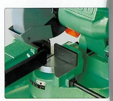
Maximum piece support even for the shortest cut lengths
