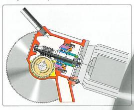
DOUBLE BALL BEARING SUPPORT OF BLADE DRIVE. Minimises vibration for superior cutting performance and longer machine life.
