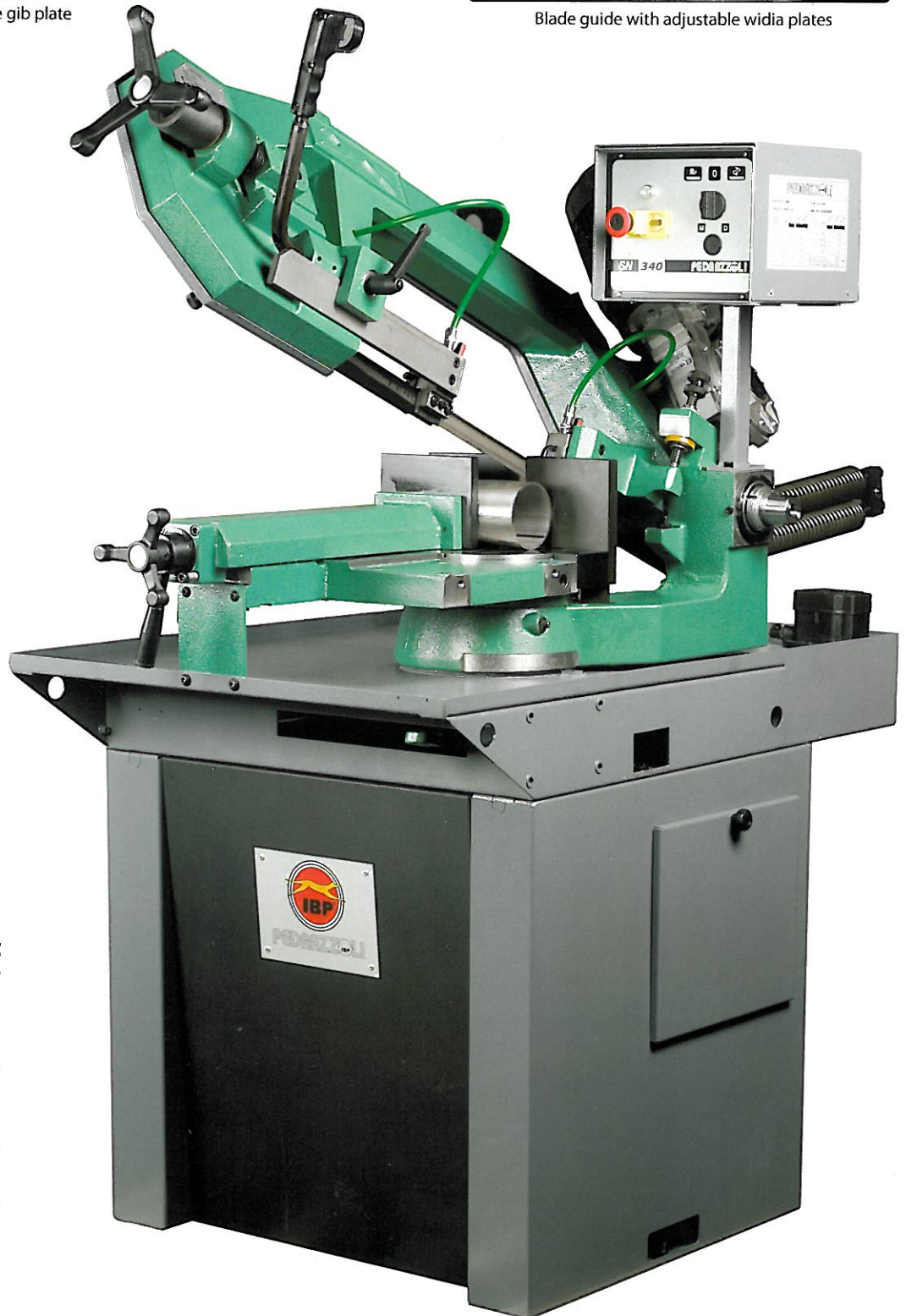
(*) Retractable vice shoulders to reach maximum cutting capacity (340 x 180 mm). Easy reading of engraved graduated scale
