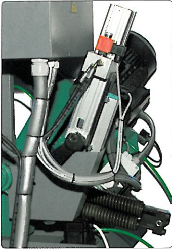
Hydraulic cylinder group for bow movement
